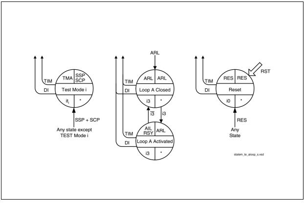
Figure 68 State Transition Diagram of Unconditional Transitions (TE)
