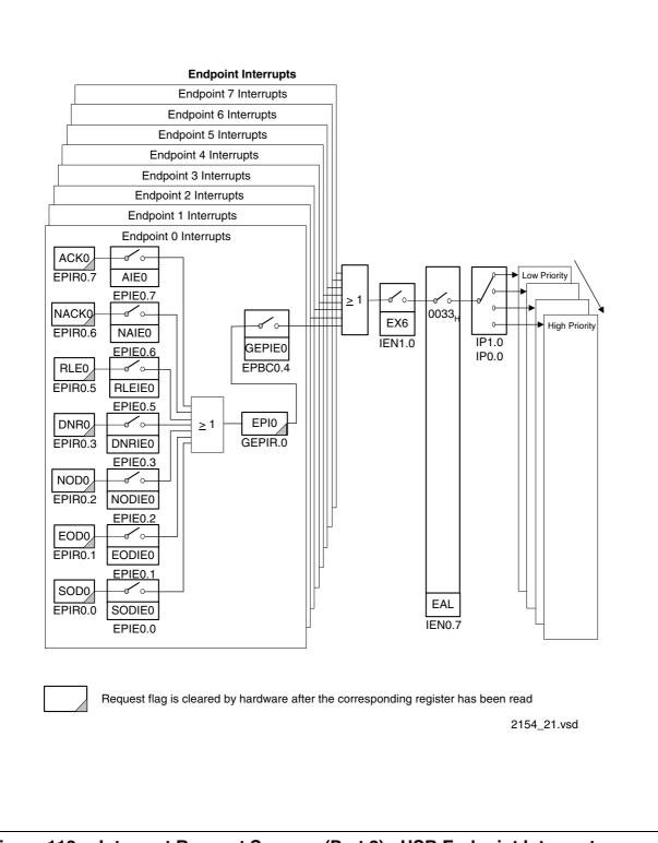
Figure 112 Interrupt Request Sources (Part 2) - USB Endpoint Interrupts
