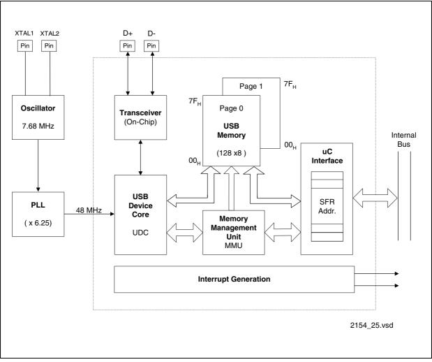
Figure 24 USB Module Block Diagram
