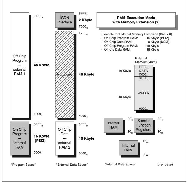
Figure 123 Firmware Execution in RAM - Example with One 64K Memory
