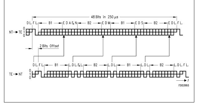
Figure 53 Frame Structure at Reference Points S and T (ITU I.430)
