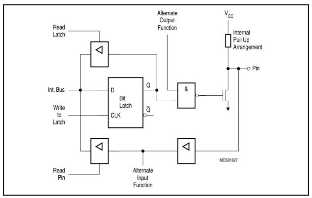
Figure 17 Port Alternate function
