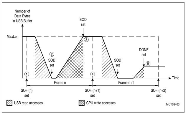
Figure 29Single Buffer Mode : Standard USB Read Access
