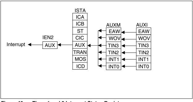
Figure 46 Timer 1 and 2 Interrupt Status Registers
