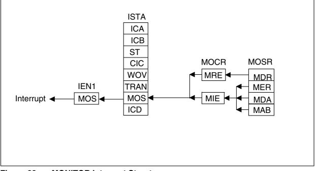
Figure 92 MONITOR Interrupt Structure
