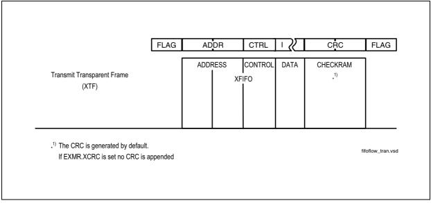
Figure 107 Transmit Data Flow
