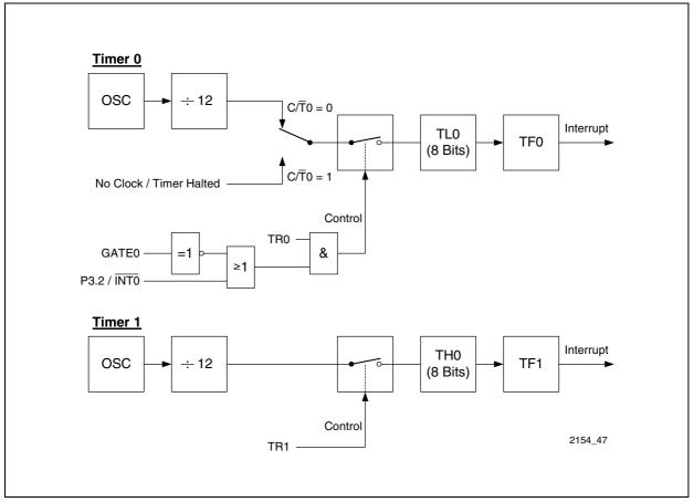
Figure 22 Timer Mode 3: Two 8-Bit Timers
