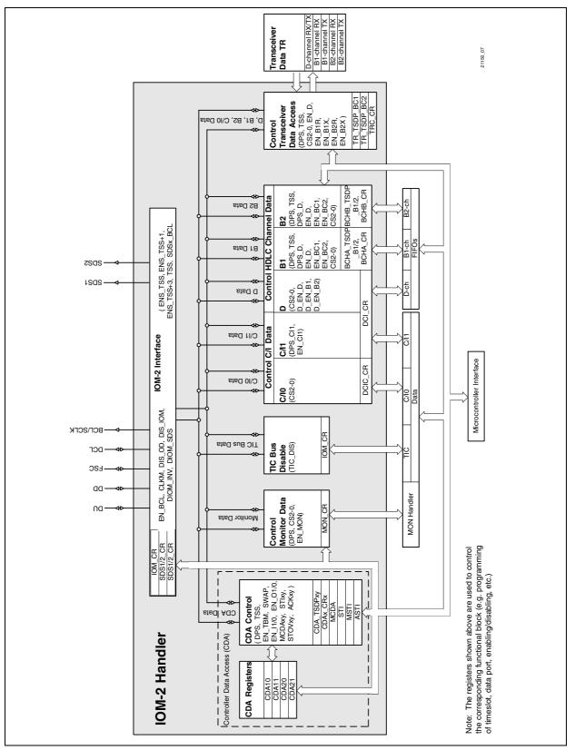
Figure 73 Architecture of the IOM Handler (Example Configuration)
