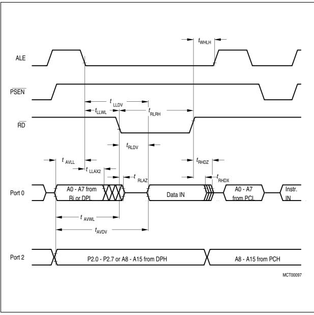
Figure 146 Data Memory Read Cycle - Emulation Mode
