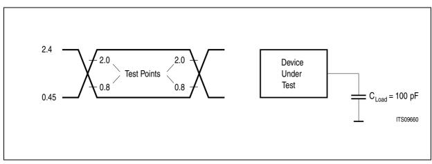
Figure 139 Input/Output Waveform for AC Tests
