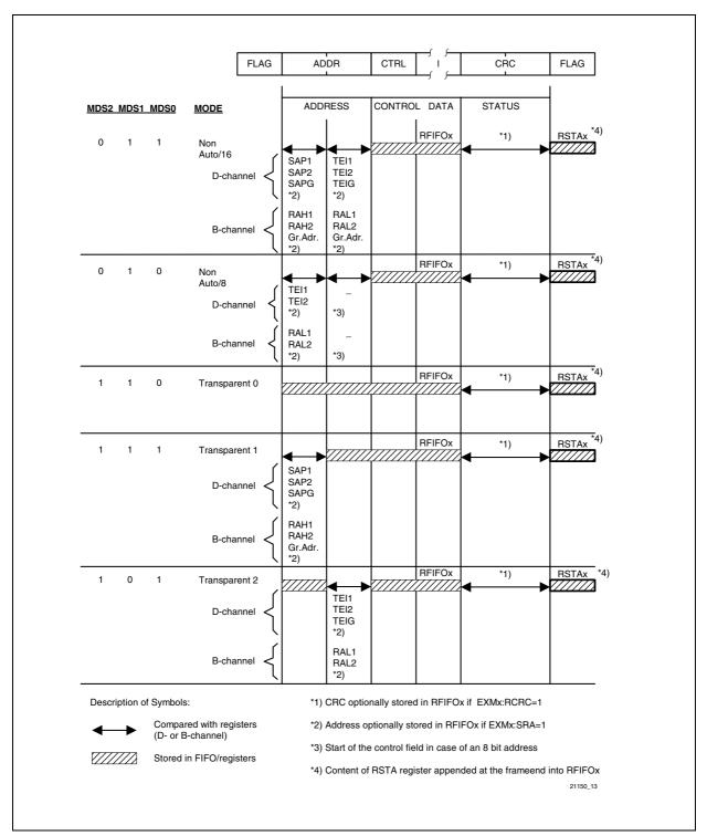
Figure 104 Receive Data Flow
