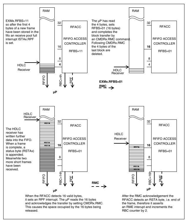
Figure 101 RFIFO Operation
