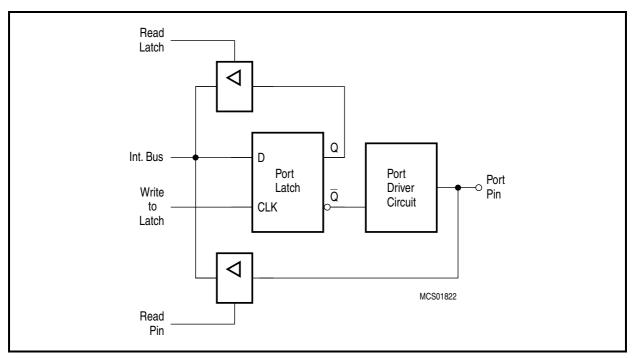
Figure 16 Basic Structure of a Port
