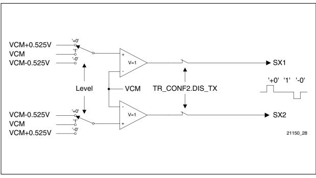
Figure 58 Equivalent Internal Circuit of the Transmitter Stage
