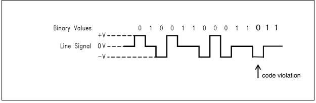
Figure 52 S/T -Interface Line Code
