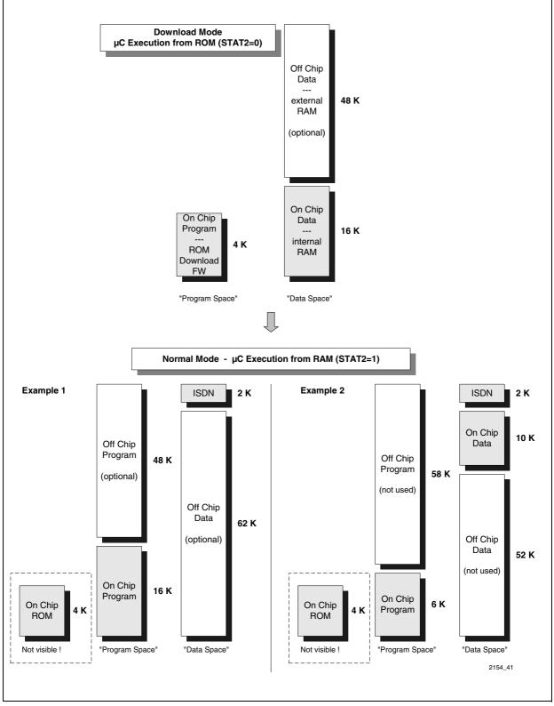
Figure 14 Switching from Download Mode to Operational Mode
