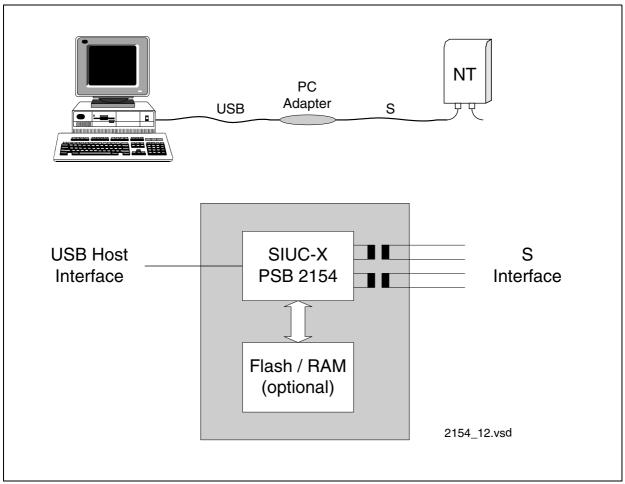
Figure 2 ISDN PC Adapter for S Interface
