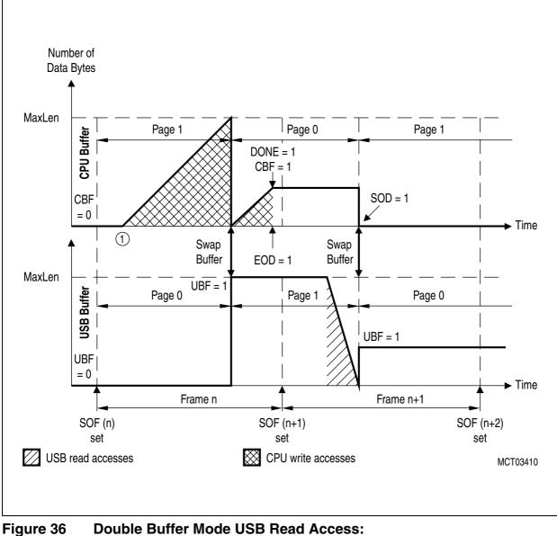
Double Buffer Mode USB Read Access: Data Length greater than Packet Length (MaxLen)
