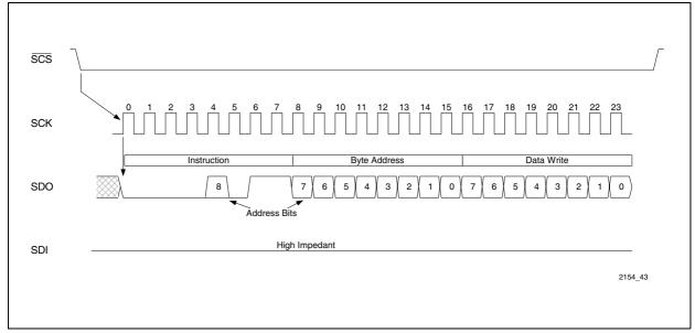
Figure 134 SPI Write Access
