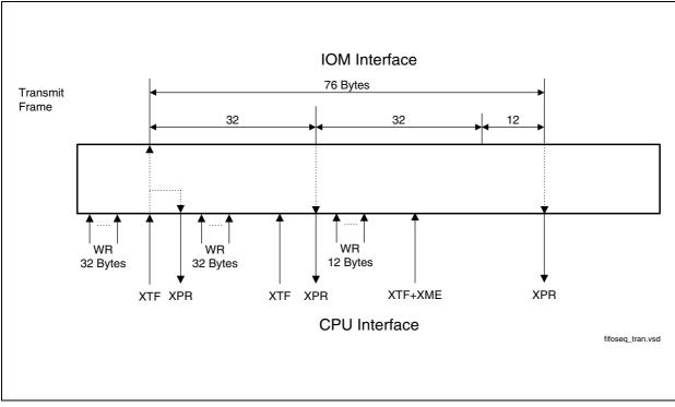
Figure 106 Transmission Sequence Example
