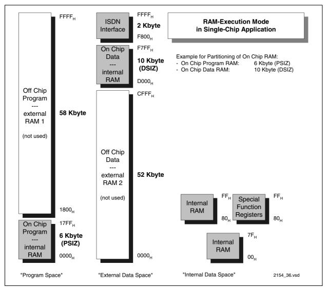
Figure 120 Firmware Execution in RAM - Single Chip Mode
