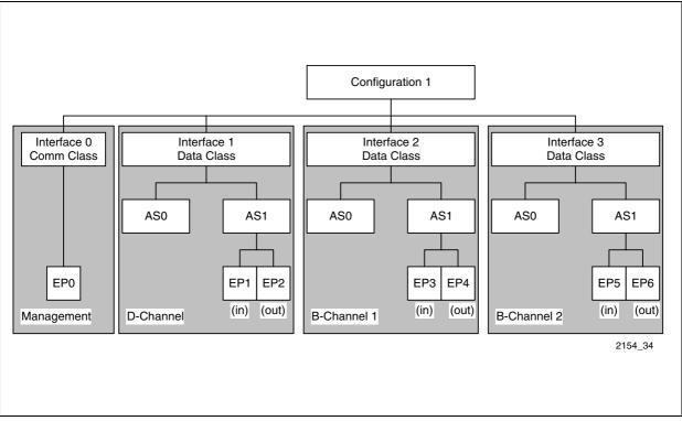
Figure 129 USB Configuration in CDC Mode
