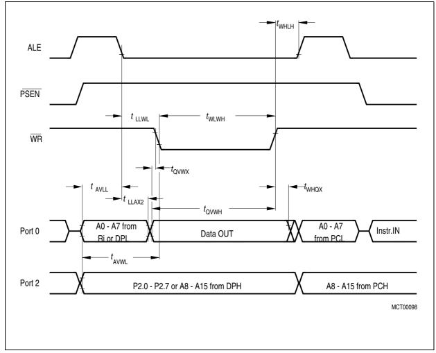
Figure 147 Data Memory Write Cycle - Emulation Mode
