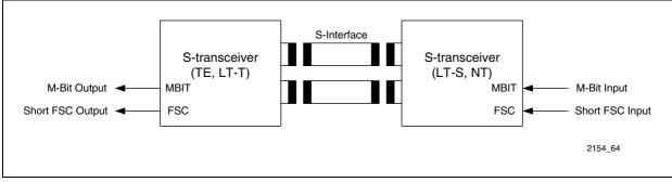
Figure 54 Multiframe Synchronization using the M-Bit
