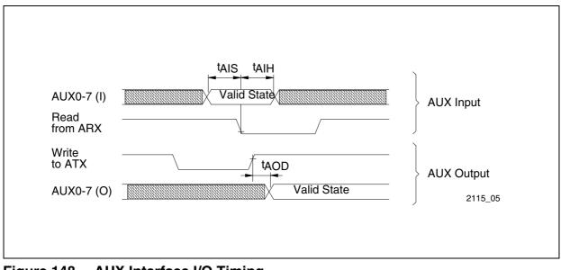
Figure 148 AUX Interface I/O Timing
