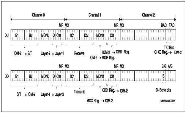
Figure 72 IOM-2 Frame Structure in Terminal Mode
