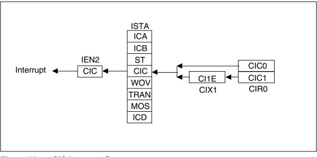
Figure 93 CIC Interrupt Structure
