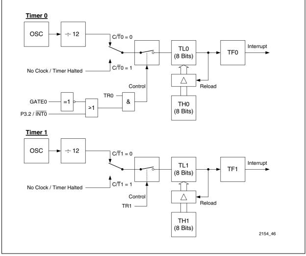
Figure 21 Timer Mode 2: 8-Bit Timer with Auto-Reload
