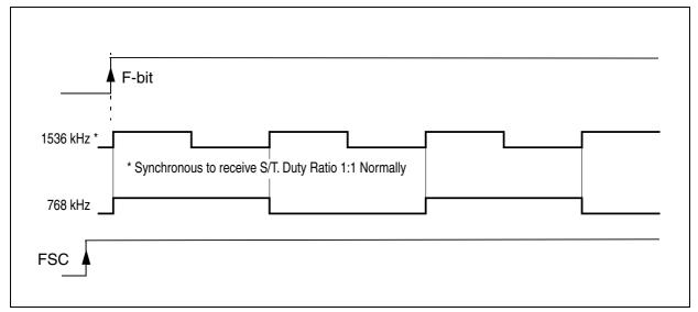
Figure 131 Phase Relationships of SIUC-X Clock Signals
