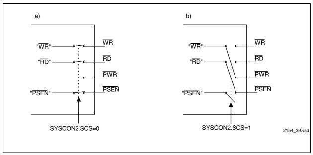
Figure 13 Switching of Read/Write Strobe Signals for Separate Memory
