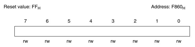
In order to enable ISDN interrupt generation to the microcontroller, the ISTA\_INIT register must be programmed to  $00_H$  after reset. After that this register should not be changed any more.
