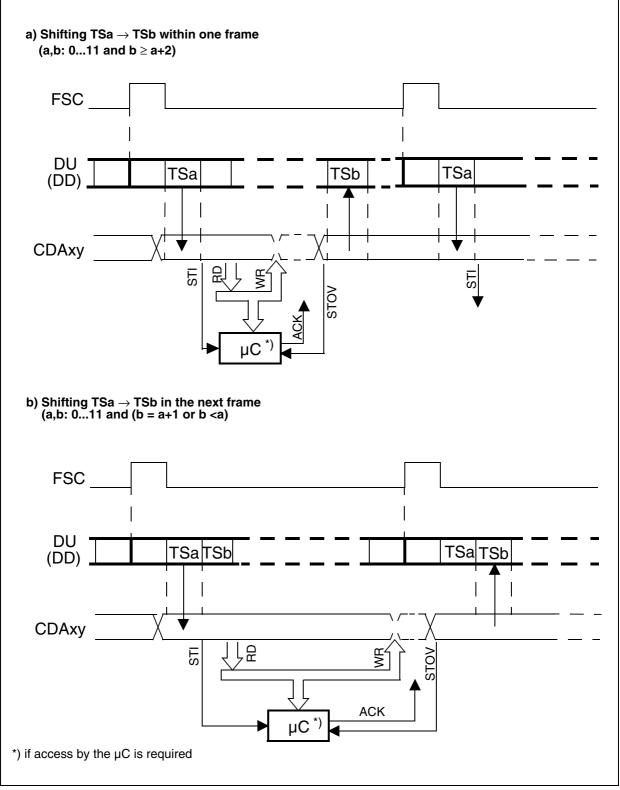
Figure 77 Data Access when Shifting TSa to TSb on DU (DD)
