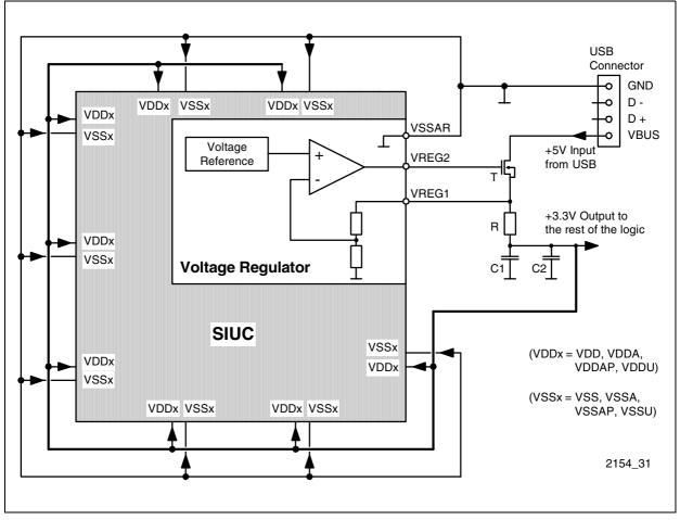
Figure 135 External Circuitry of the Voltage Regulator
