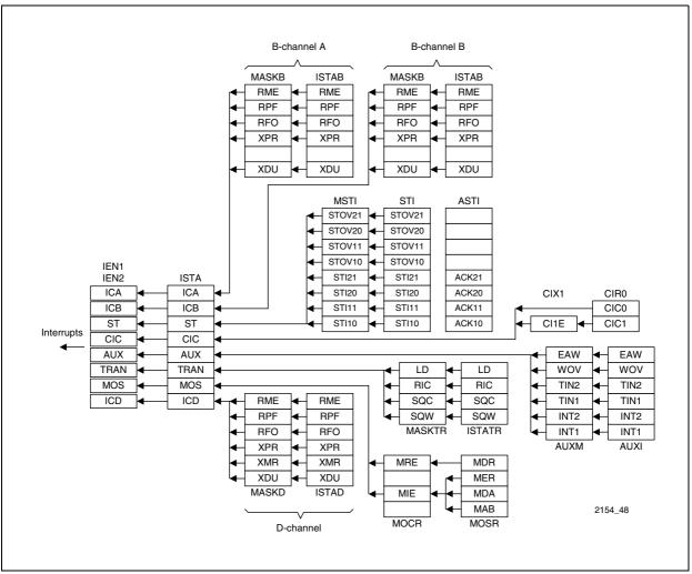
The structure of the ISDN interrupt status registers is shown in Figure 115.
