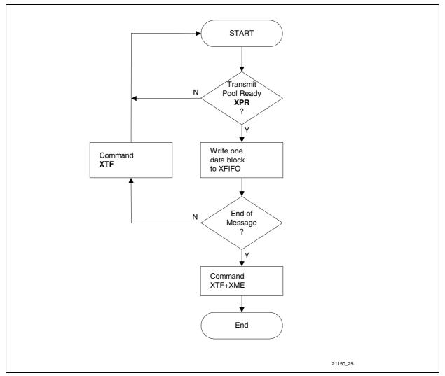
Figure 105 Data Transmission Procedure
