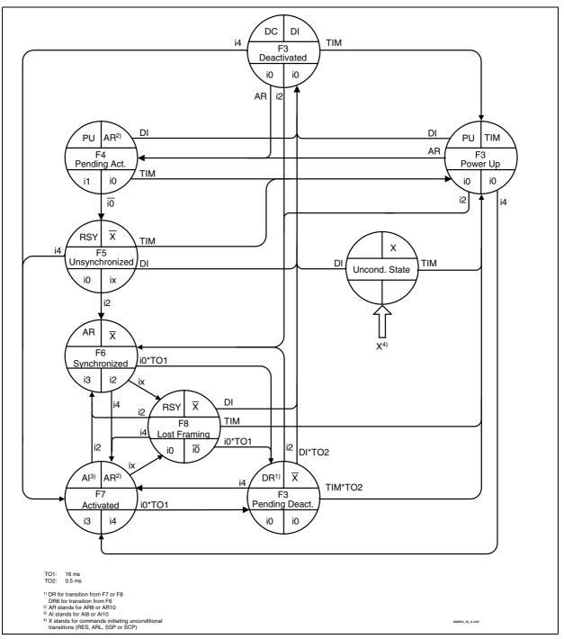
Figure 67State Transition Diagram (TE)
