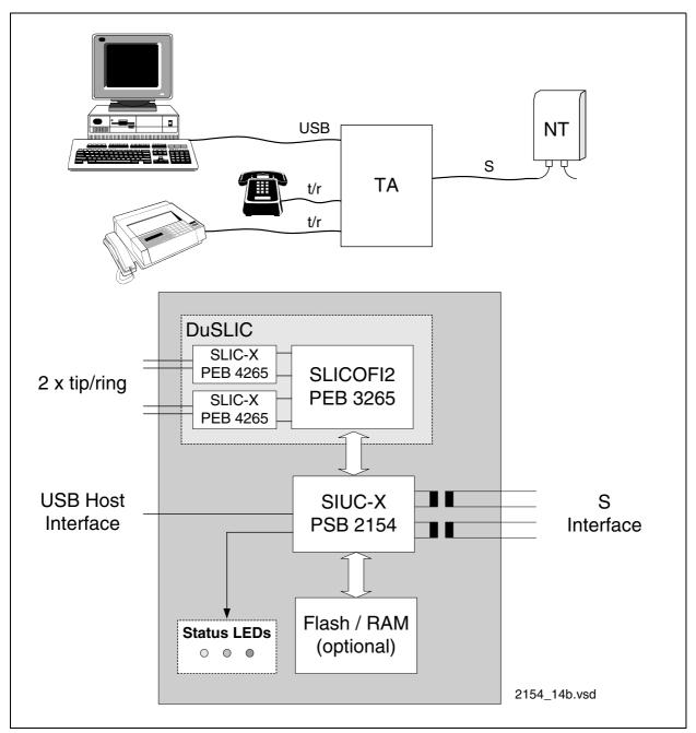
Figure 5 ISDN Stand-alone Terminal with POTS Interface
