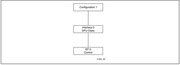
Figure 127 USB Configuration in DFU Mode
