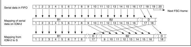
Figure 84 Mapping of Bits from IOM-2 to S
