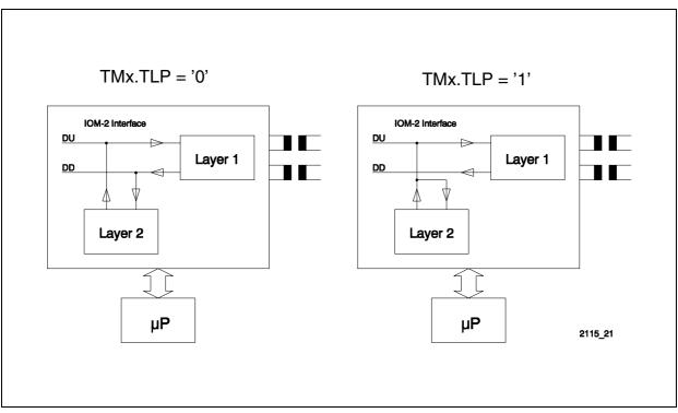
Figure 109 Layer 2 Test Loops
