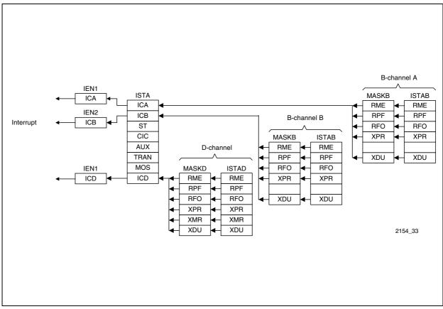
Figure 108 Interrupt Status Registers of the HDLC Controllers
