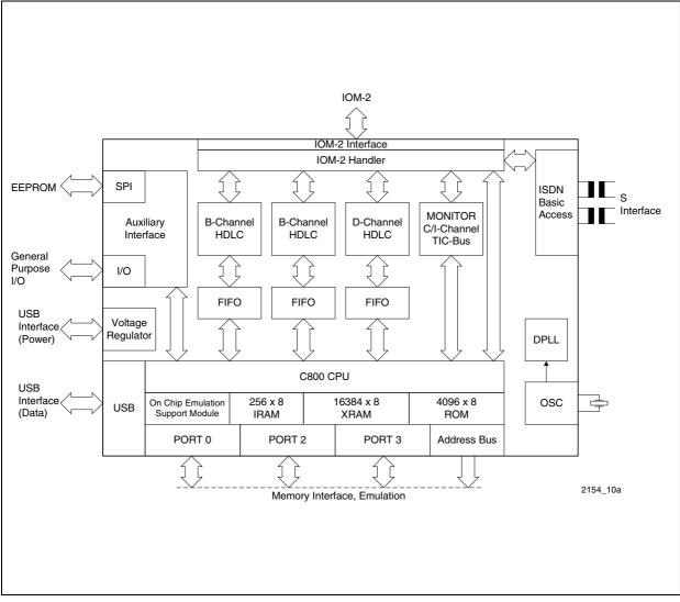
Figure 6 Block Diagram
