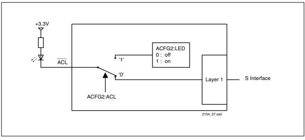
Figure 50 ACL Configuration
