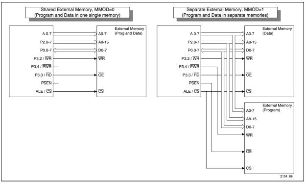
Figure 11 Shared and Separate External Memory Expansion
