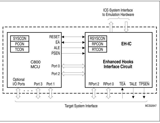
Figure 18 Basic C800 MCU Enhanced Hooks Concept Configuration
