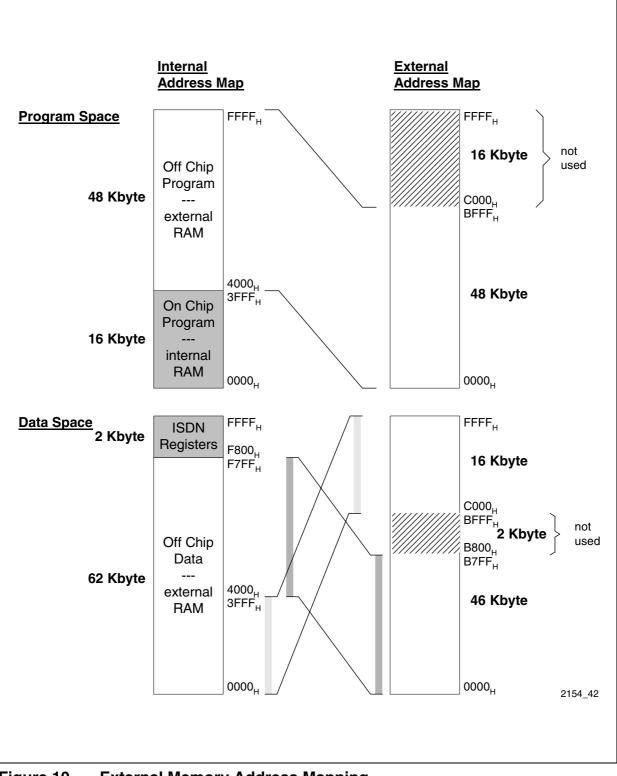
Figure 10 External Memory Address Mapping
