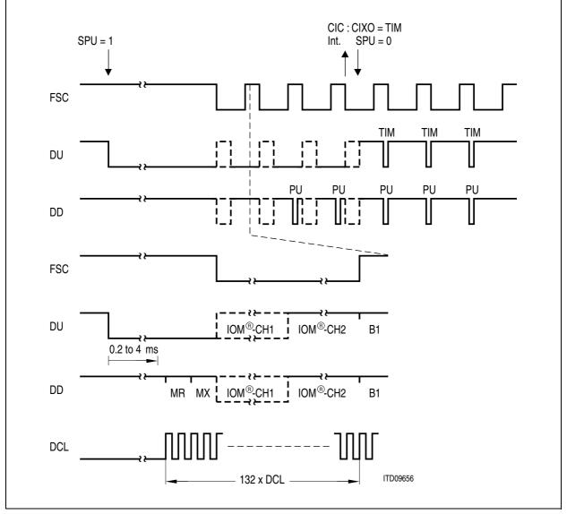
Figure 100 Activation of the IOM-2 interface
