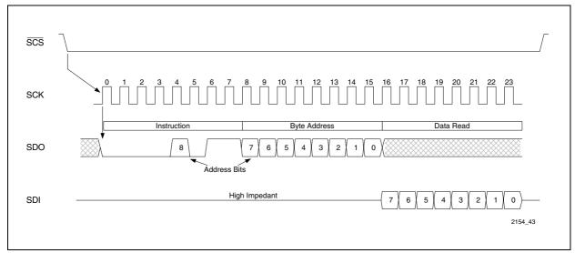
Figure 133 SPI Read Access
