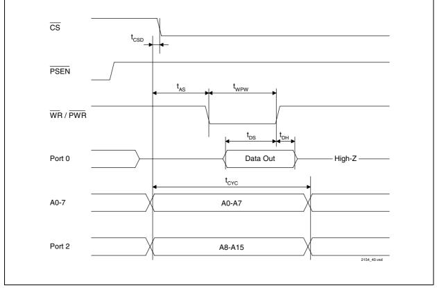
Figure 144 Data Memory Write Cycle - Normal Mode
