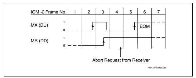
Figure 89 Monitor Channel, Transmission Abort requested by the Receiver
