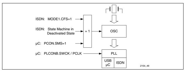
Figure 136 Clocks in Suspend Mode
