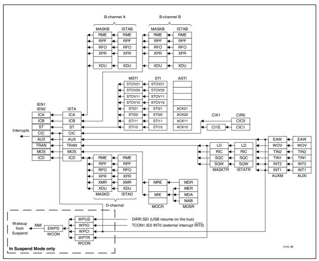
Figure 116 Wakeup Sources in Suspend Mode
