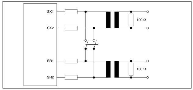
Figure 64 External Loop at the S/T-Interface
