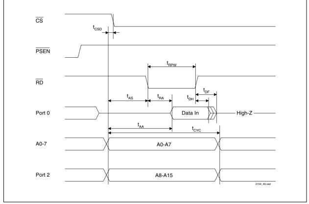
Figure 143 Data Memory Read Cycle - Normal Mode
