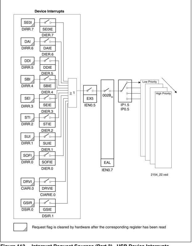
Figure 113 Interrupt Request Sources (Part 3) - USB Device Interrupts
